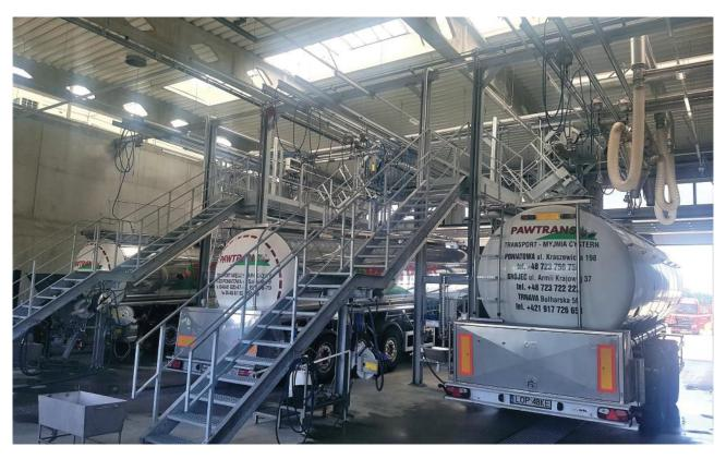
OMZ manufactures and installs internal washing systems for tanks, whether they are used for the transport of food and / or chemical products.
