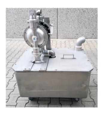
In essence, this is a trolley-mounted tank in stainless steel with a capacity of 250 liters, inside which a special liquid for pickling, which is normally found on the market, will be placed.
